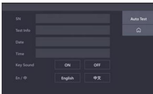
**Auto Test:** Can self-test again after powering on. The self-test items will be displayed one by one in Test Info
