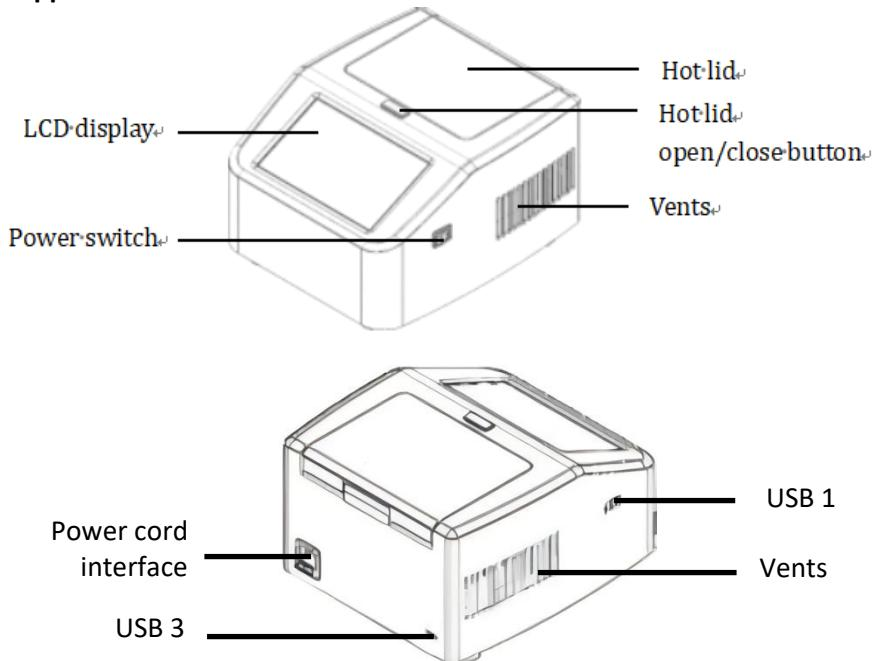
**LCD display:** parameter display, program operation display and parameter setting.
