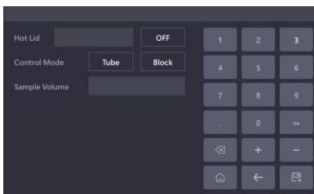
**Hot lid:** It is turned on by default. The default temperature is 110°C. You can also directly input the hot lid temperature that needs to be set. The setting range is room temperature - 110°C. After clicking off, the hot lid will be closed. If the Block temperature is lower than 30°C, the hot lid will be turned off by itself.
