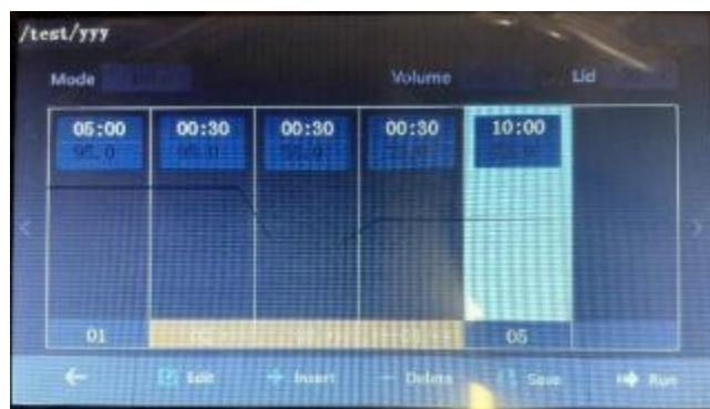
① **Pre-denaturation 95°C, 5 minutes:** In column 01, enter 95 for TempL, TempH will automatically input 95, enter 500 for Time setting, and the STEP setting is completed.
