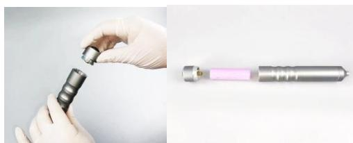
C) Hold the barrel of the grinder with your hands and insert the grinding rod of the required size into the grinder joint in the direction shown in the figure.
