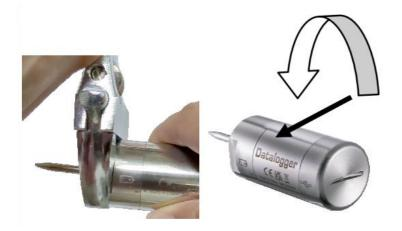
3. Remove the old battery and O-ring, then install the new battery and O-ring. Ensure the battery is oriented correctly according to the polarity markings.
