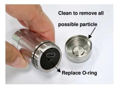
To close, rotate the cover clockwise until it aligns with the marking.
