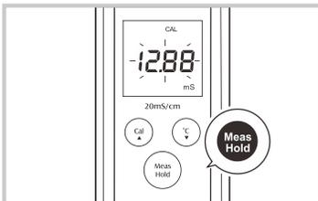
5. Press the **Meas** key, the calibration value will automatically flash 3 times. The tester returns to the measurement mode. Calibration is completed.
