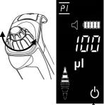
② Press **Parameter Knob** to switch the pipette off.
