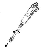
③ Separate the seal gasket and O ring from piston cover.
